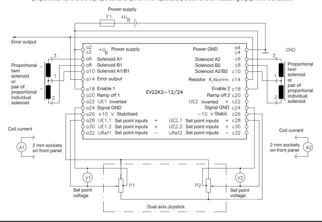
The arrangement on page 8 applies to the most used circuitry for EV22K2-12/24 where joy-sticks with wiper are used (see also example circuit 1 in sect. 6.1).
